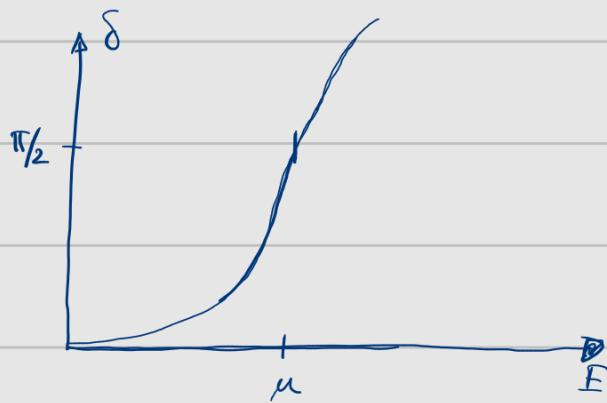
typical behaviour of the phase shift in the presence of a resonance-
