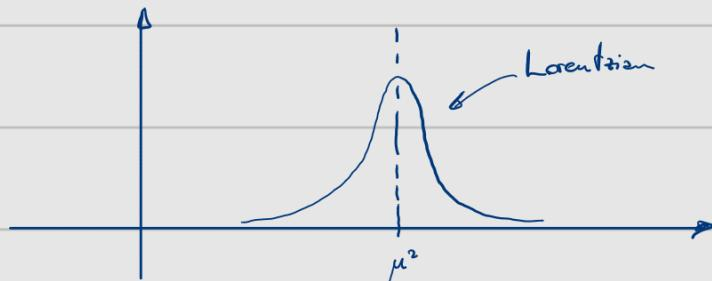
$k^2 - \mu^2 = \pm \mu \Gamma \rightarrow$  full width at half maximum is  $2\mu \Gamma$ , but if we convert the expression to depending on energy in the rest frame of the decaying particle:
